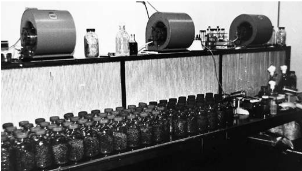
Paul Stamets's 12-foot-long laminar flow bench designed for commercial cultivation. Simple, but effective.
