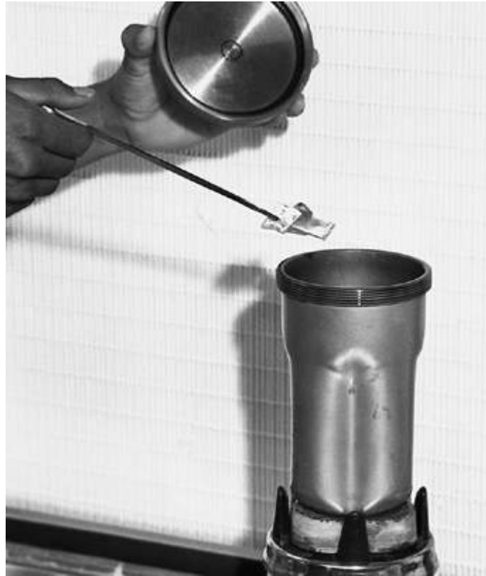
Inoculating an Eberbach stirrer with agar wedges of mycelium in airstream of laminar flow hood.
