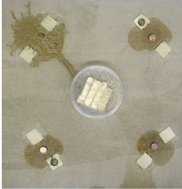
FIGURE 120 Here, when an extract of a presporulating entomopathogenic mycelium grown on rice is placed onto cellulose, termites tunnel to it, ignoring three nontreated controls.
