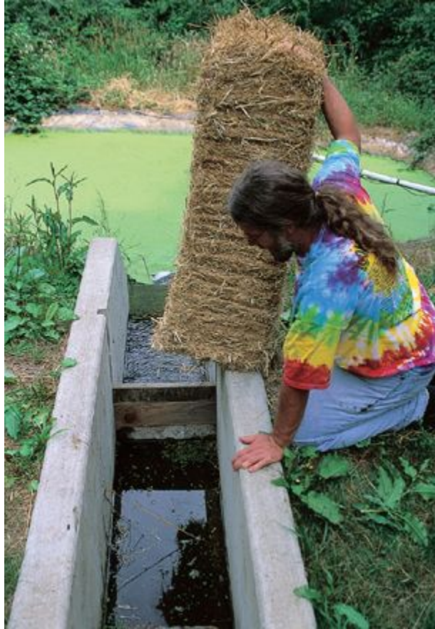
FIGURE 72 This mycofiltration test chamber, sized to fit a bale of straw, myceliated or not, can be sectioned off, and samples of water can be taken both upstream and downstream.
