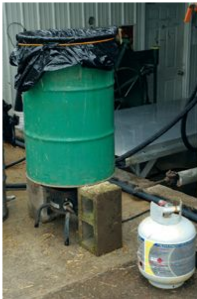
FIGURE 170 Using a food-grade steel drum and crab-pot burner for hot-water or steam pasteurization of straw.
