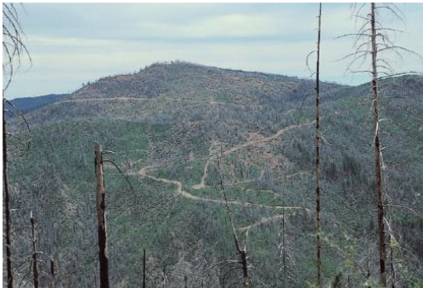
FIGURE 87 Logging roads channel silt into valleys, such as occurs along this northern California hillside etched with zigzagging logging roads.
