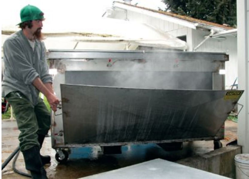
FIGURE 171 A specially designed stainless steel pasteurization chamber. Steam is injected through a port on the side. Once pasteurization is complete, the door is lowered and doubles as a ramp for unloading the straw.
