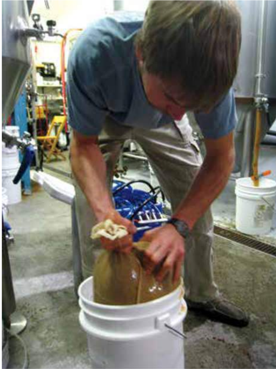
T. J. Daly, the head brewer at Smuggler Joe's in Telluride, Colorado, strains a batch of medicinal mushroom extracts into a sanitized bucket to remove the grain solids before adding them to the kegs. The director of the festival, Scott Koch, helped design the formula and assisted with the brewing.
