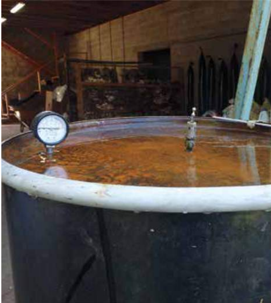
A 55-gallon drum can be modified to hold a few pounds of pressure using a release valve and pressure gauge. It can be used to super-pasteurize media for six hours.
