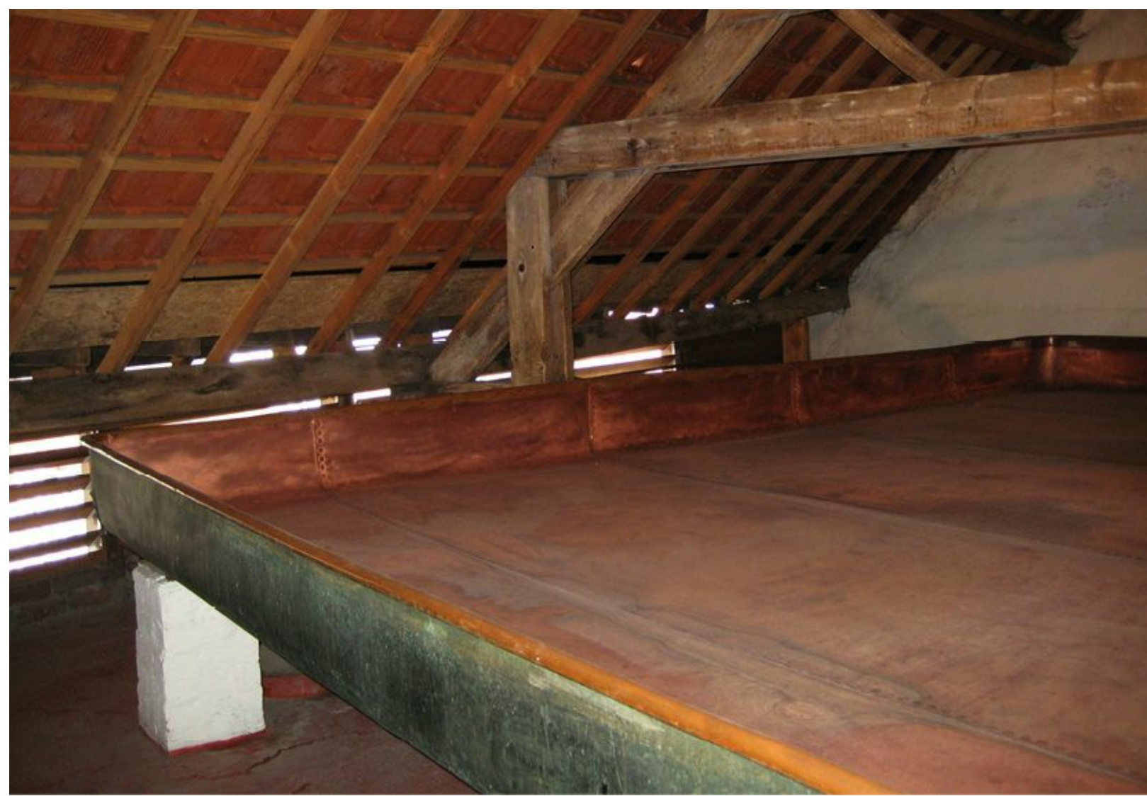
The coolship at Brewery Cantillon in Brussels, where the wort cools and collects wild yeast and bacteria from the air via its broad exposed surface.
