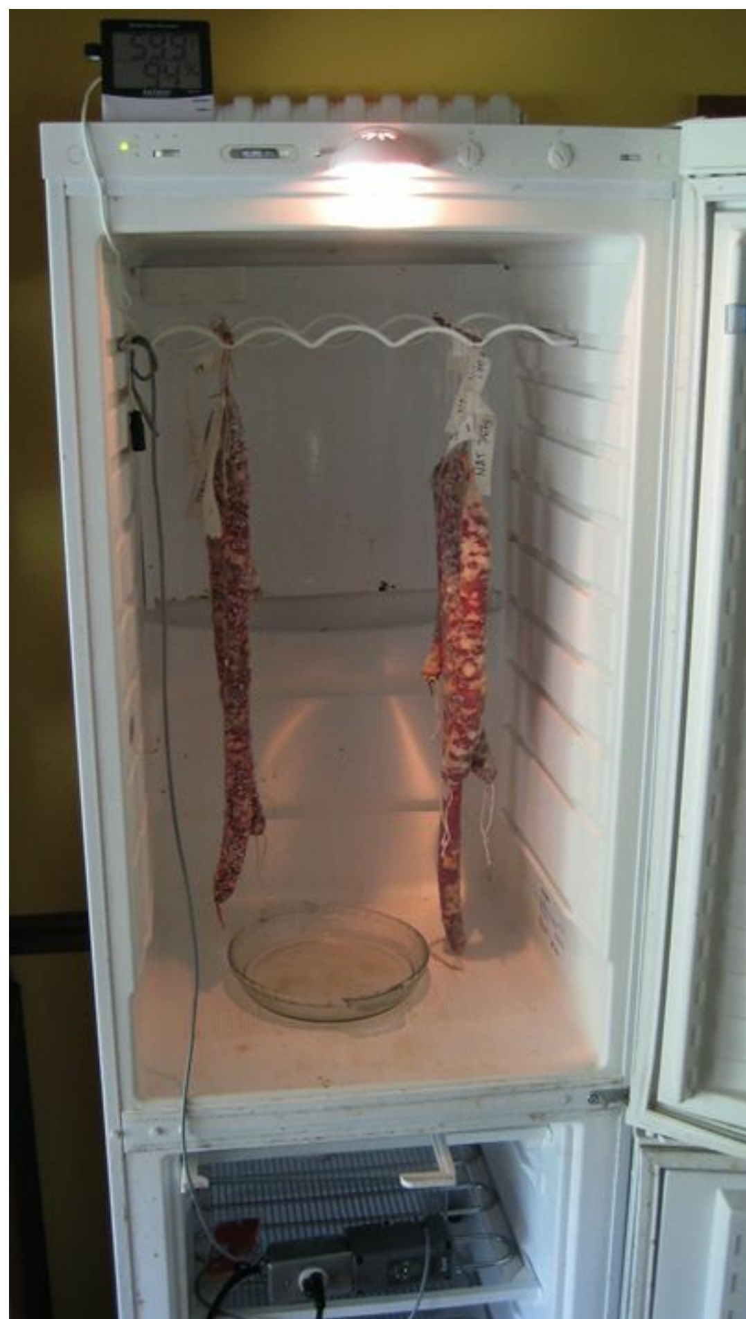
The author's salami-curing chamber, a refrigerator with an overriding temperature controller set for 57°F/14°C.
